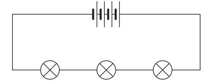
Three bicycle bulbs are connected in series. They are then connected to a four-cell battery, as shown in the above diagram.
